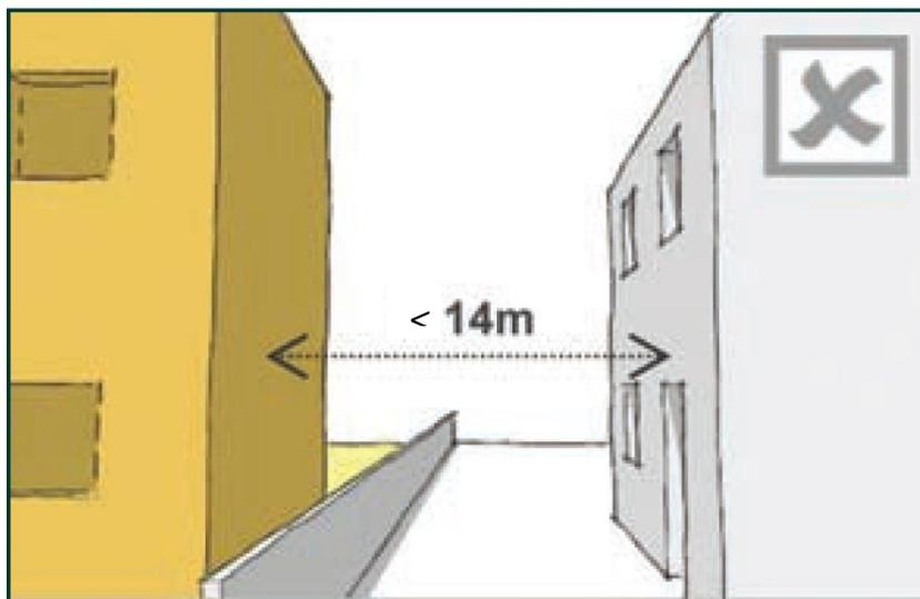
**Figure 2: Distance of 14.00 metres between a protected window and a blank two-storey wall**
