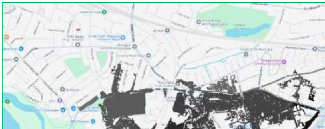
Figure 5 - Natural Resources Wales Modelled Defended 1 in 100 Year (+25%) Flood Outline: Fluvial Liswerry Pill
