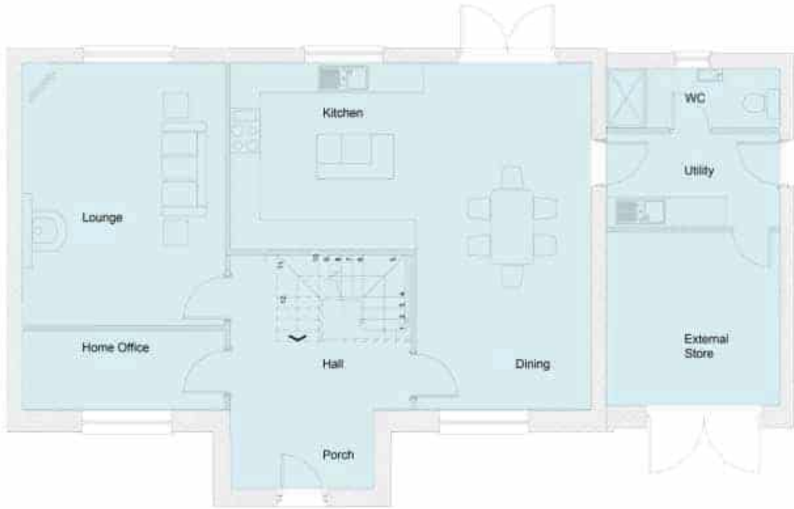
Ground Floor Plan as proposed 1:50 scale
