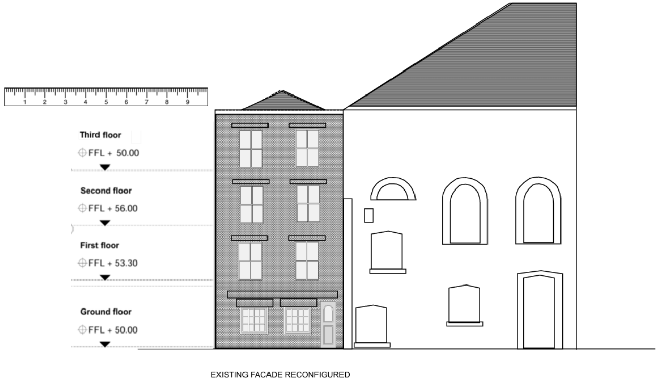
Fig 13 Rear View of developed plot, showing parapet façade with set-back roof, and neighbouring property / warehouse
