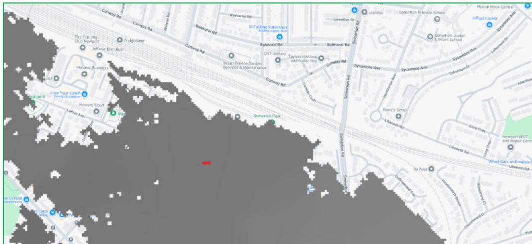
Figure 13 - Natural Resources Wales Modelled Undefended 1 in 1000 Year Flood Outline: Tidal River Usk
