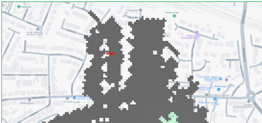
Figure 9 - Natural Resources Wales Modelled Defended 1 in 1000 Year Flood Outline: Tidal River Usk
