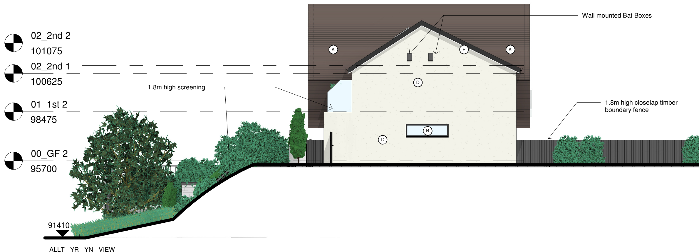
West (Side) Elevation 1 : 125
