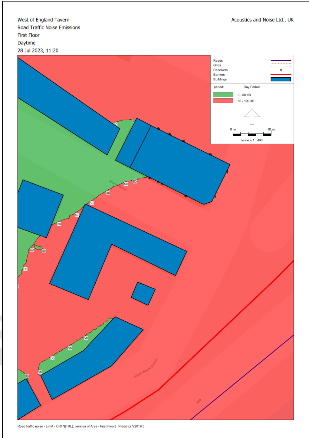
Figure 8 – Road Traffic Noise Emissions, First Floor, Daytime
