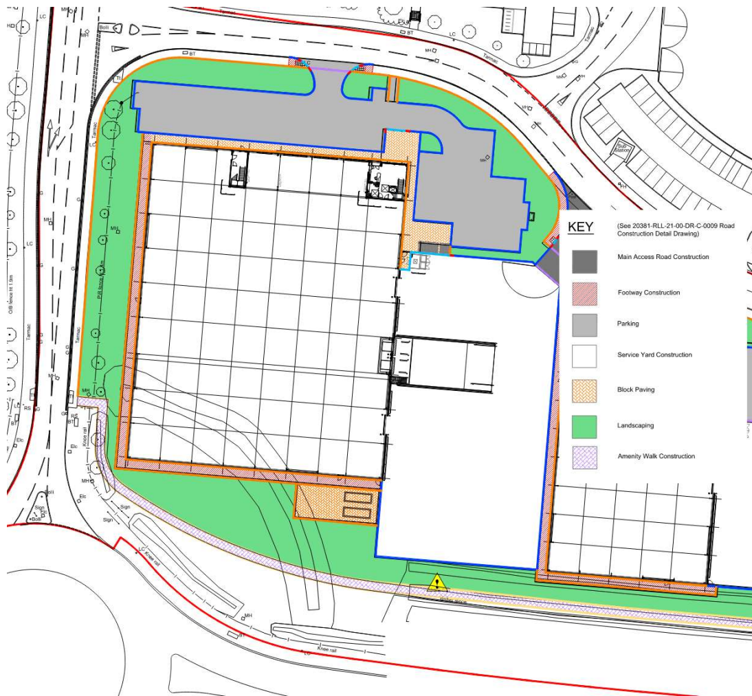
Figure 1: Existing Hardworks Layout for Unit 7
