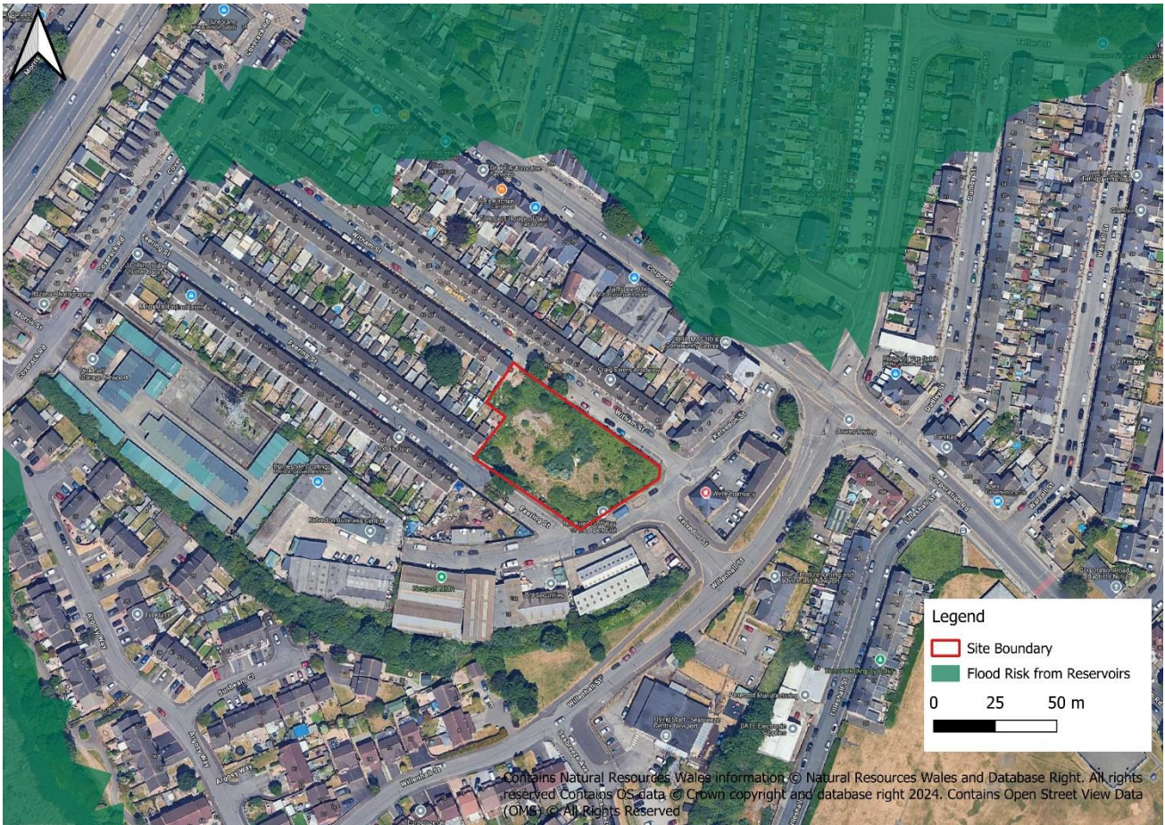
Figure 4-4 Flood Risk from Reservoirs
