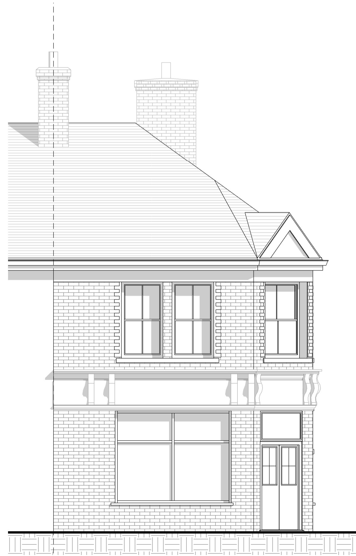
4 Existing Front Elevation(Courtybella Terrace) 1:50
