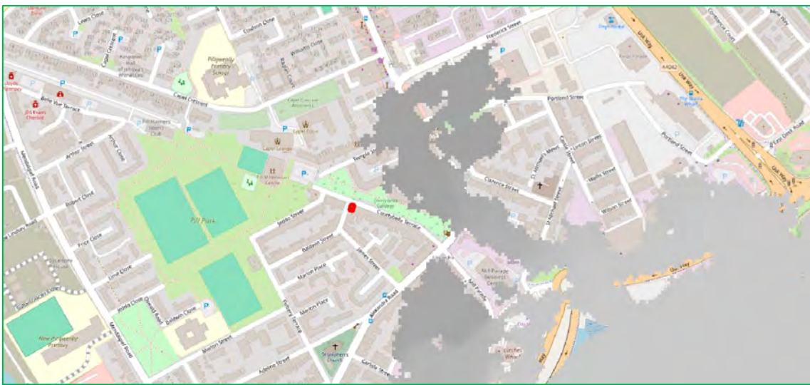
Figure 13 - Natural Resources Wales Undefended Modelled 1 in 1000 Year Flood Outline (v8 of the Newport Model)
