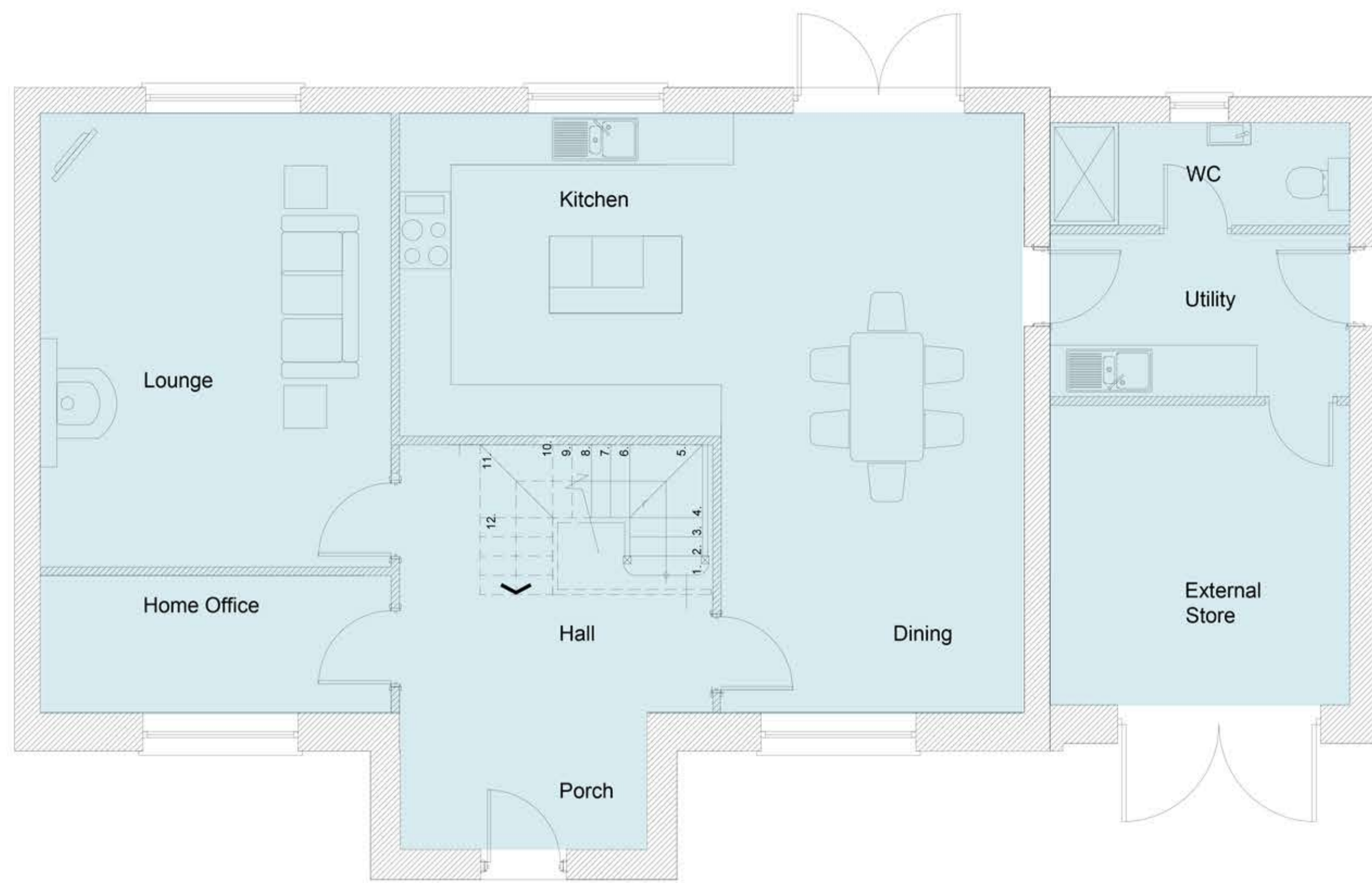
Ground Floor Plan as proposed 1:50 scale
