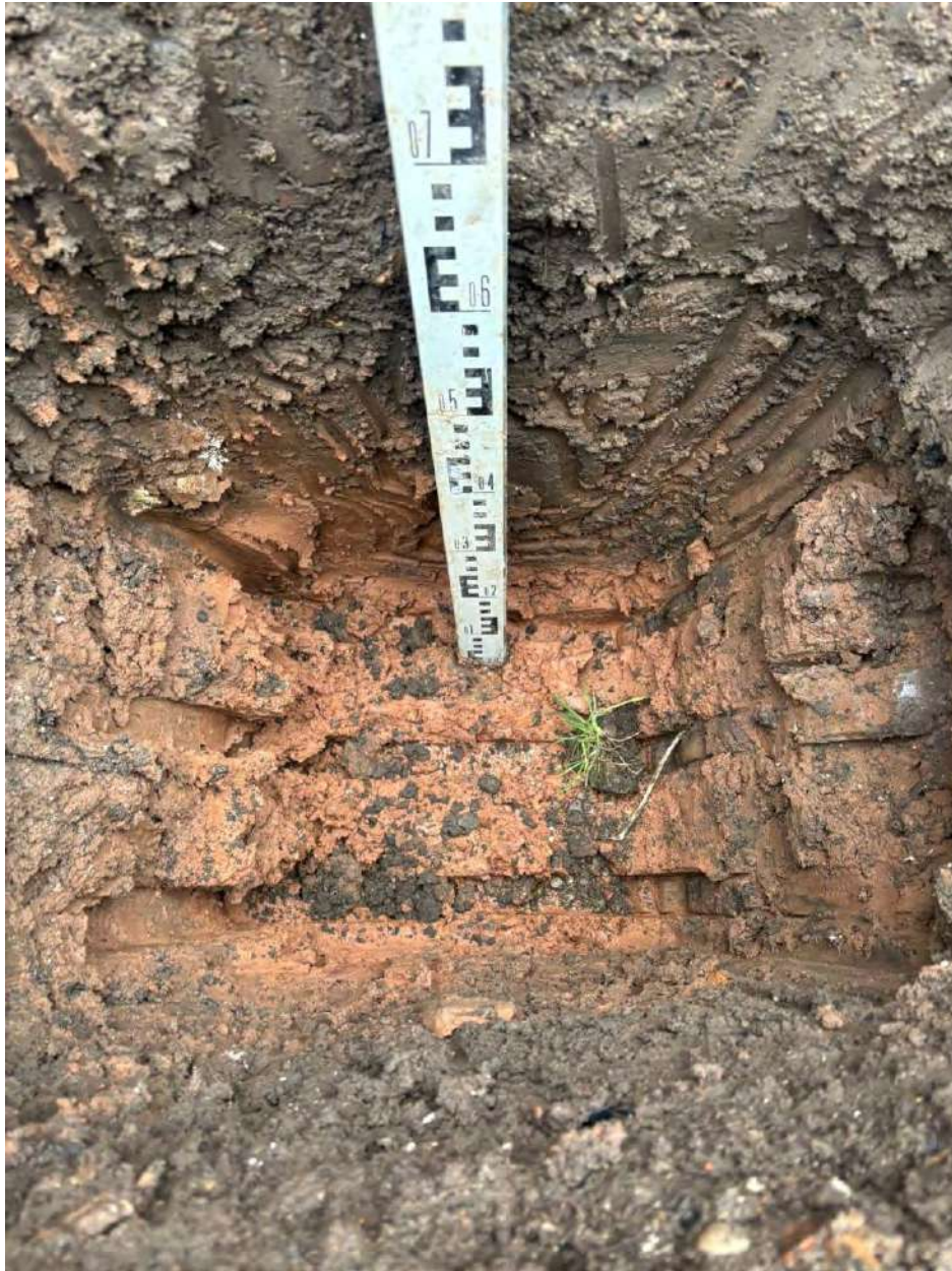
Figure 3 – TP1 showing strata in pit
