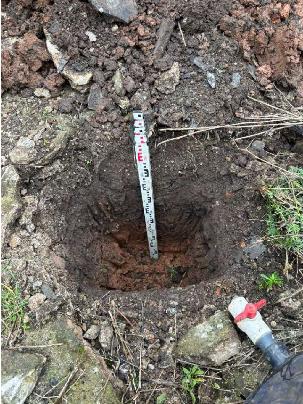
Figure 2 - Test pit 1 during excavation
