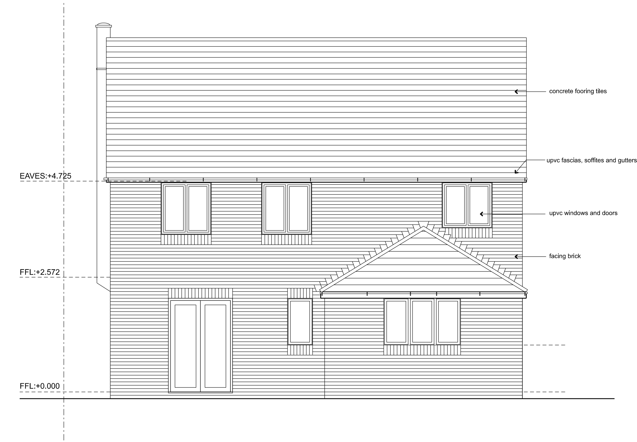
existing rear elevation
