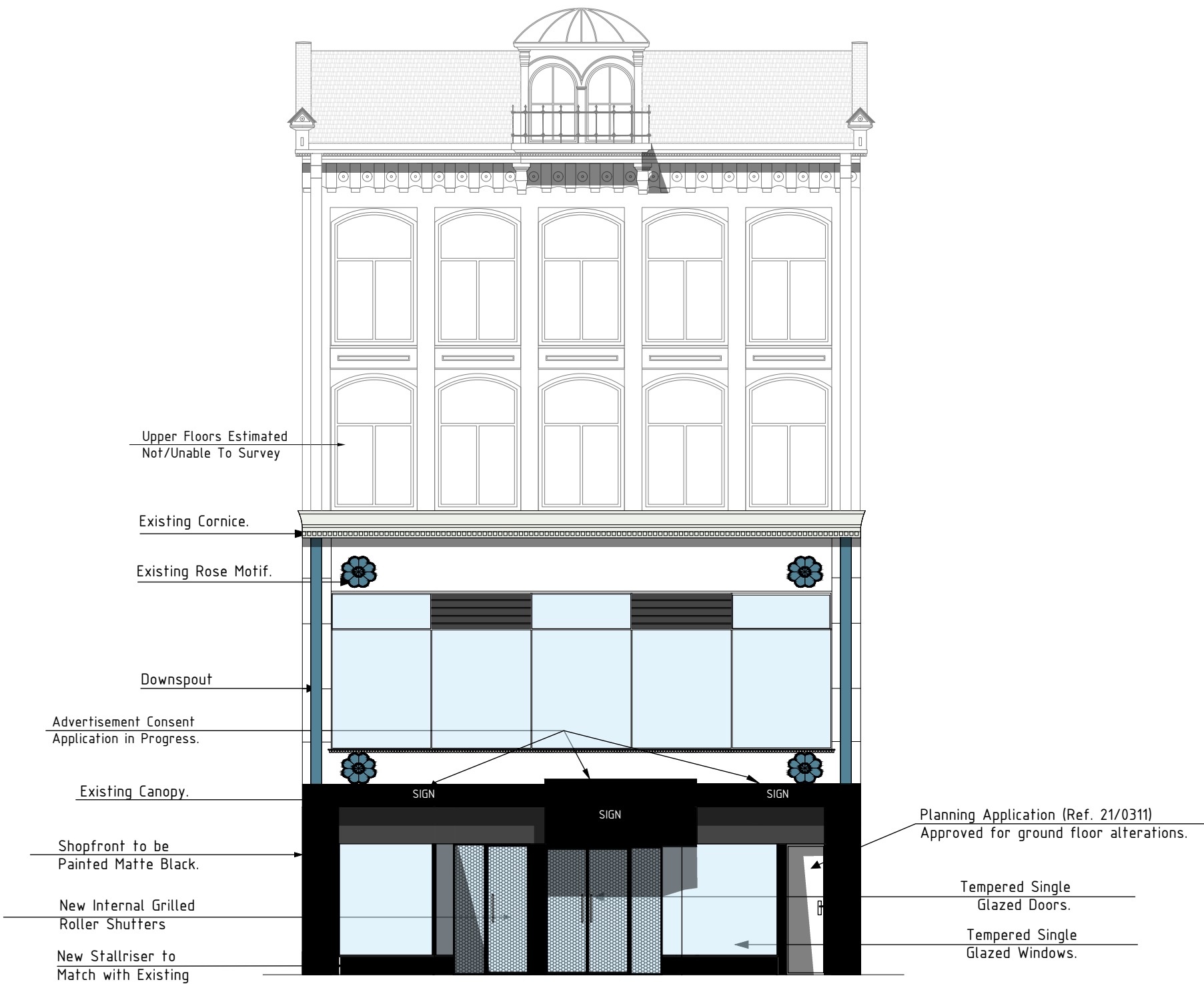
Proposed Front Elevation (Shutters Closed).
