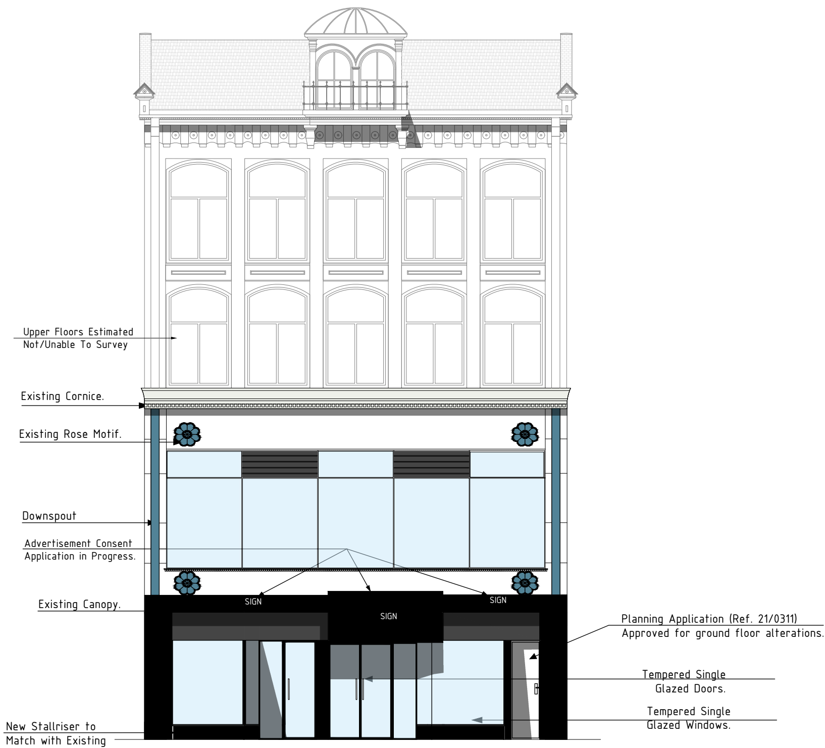
Proposed Front Elevation (Shutters Open).
