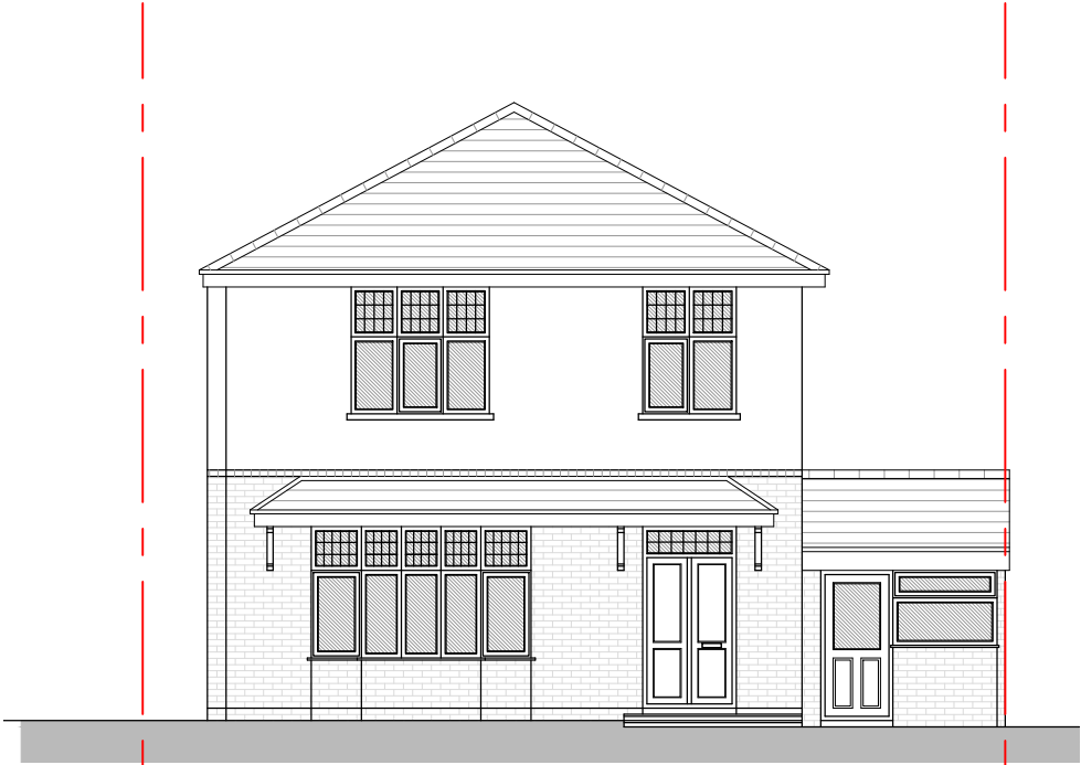
EXISTING FRONT ELEVATION 1:100 @ A3
