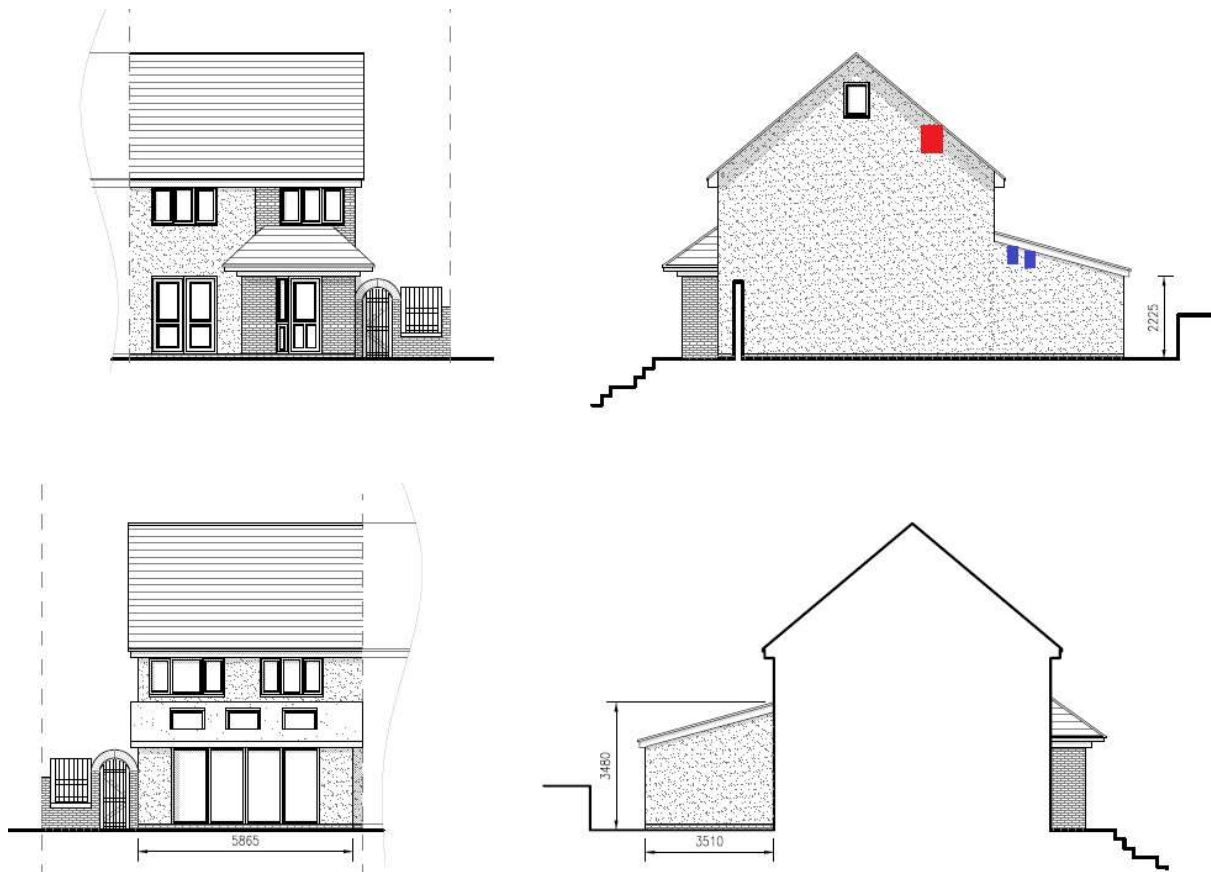
Figure 2. Position of bat (red) and bird (blue) enhancements adapted from Morris Architectural Design drawing NM/0604/2520 – 200-05
