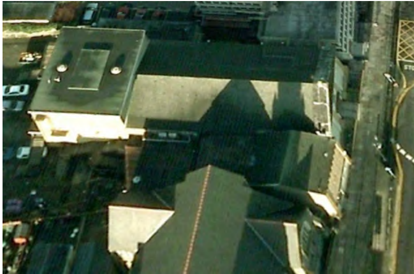
Figure A39. Roofplan showing the gable roof running parallel with the street to the south of the chapel and pitched roof on the southern building. Photo taken prior to the 2018 fire © Google Earth
