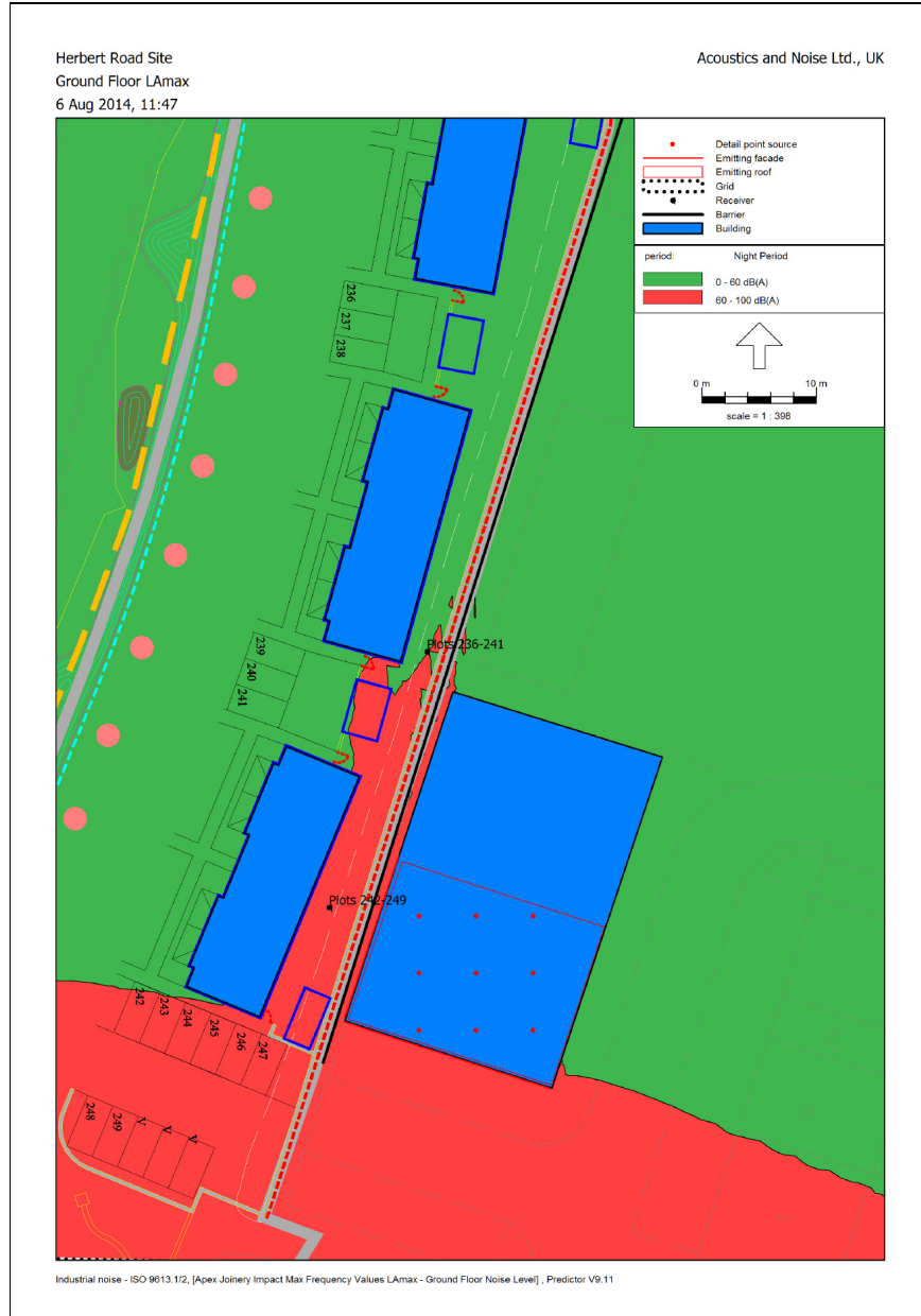
Figure 5 – Calculated External Noise Contours LAmax @1.5m
