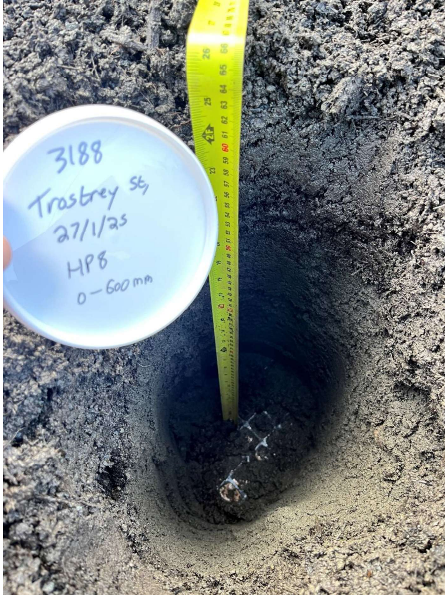
Hand pit excavated in the rear garden of Plot 8.
