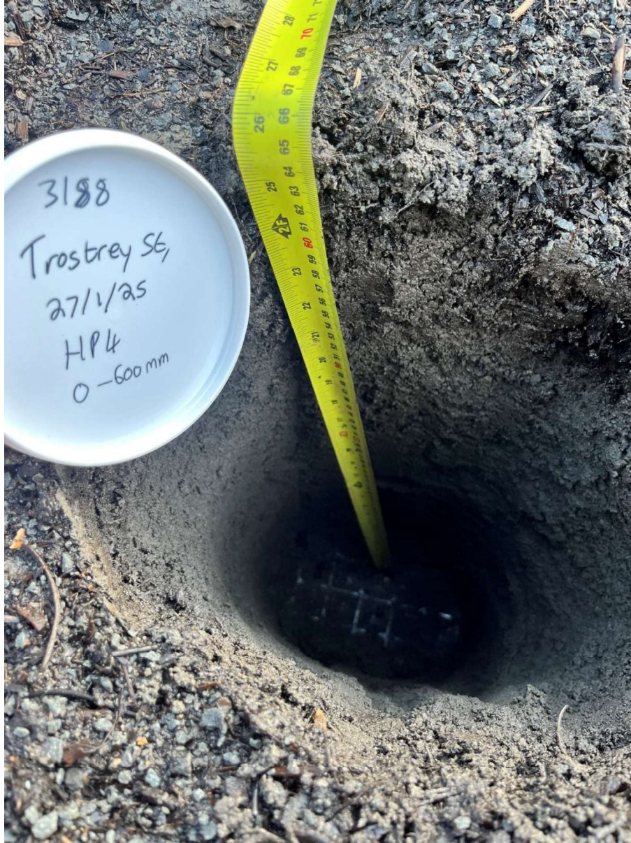
Hand pit excavated in the rear garden of Plot 4.
