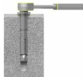
Tighten with torque wrench to Installation Torque
