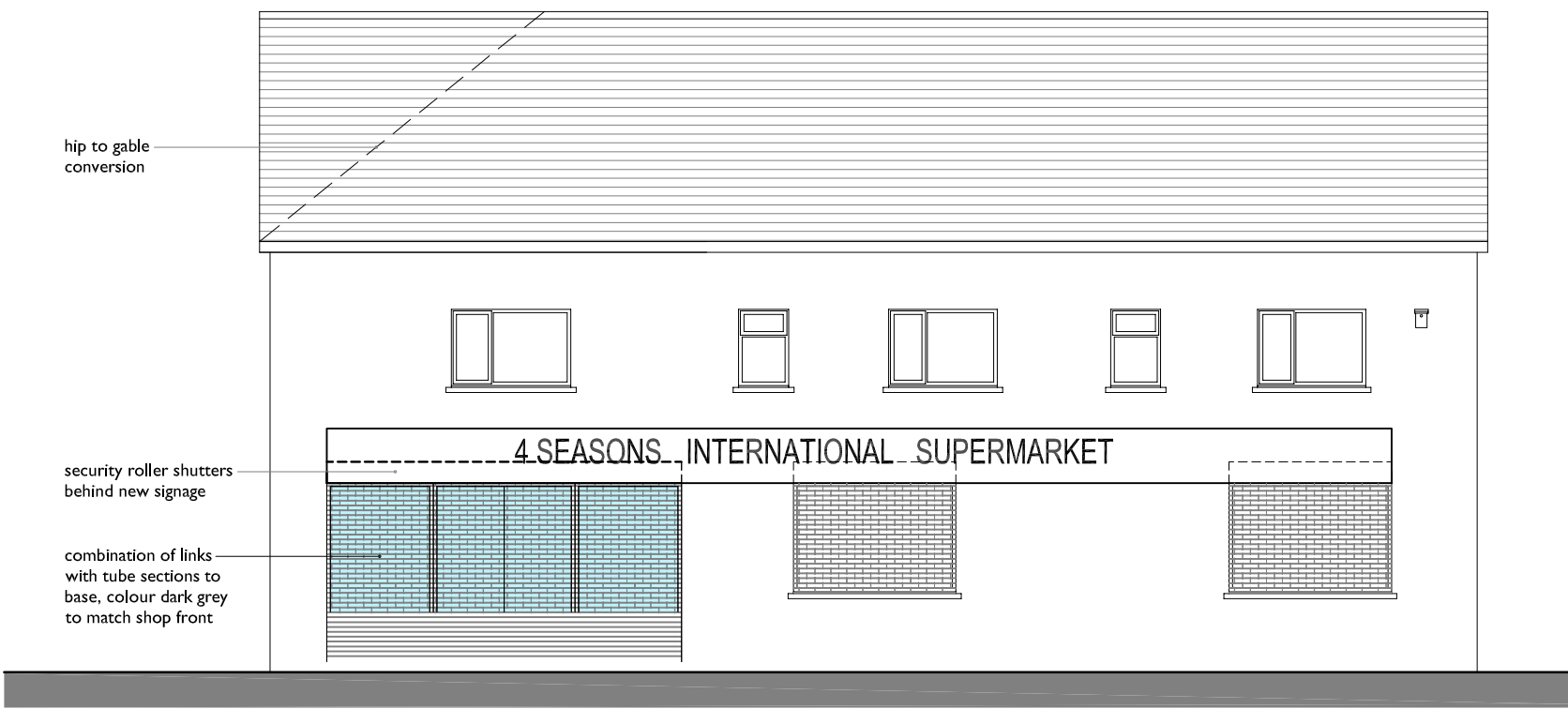
FRONT ELEVATION (WHARF ROAD) WITH SHUTTERS CLOSED
