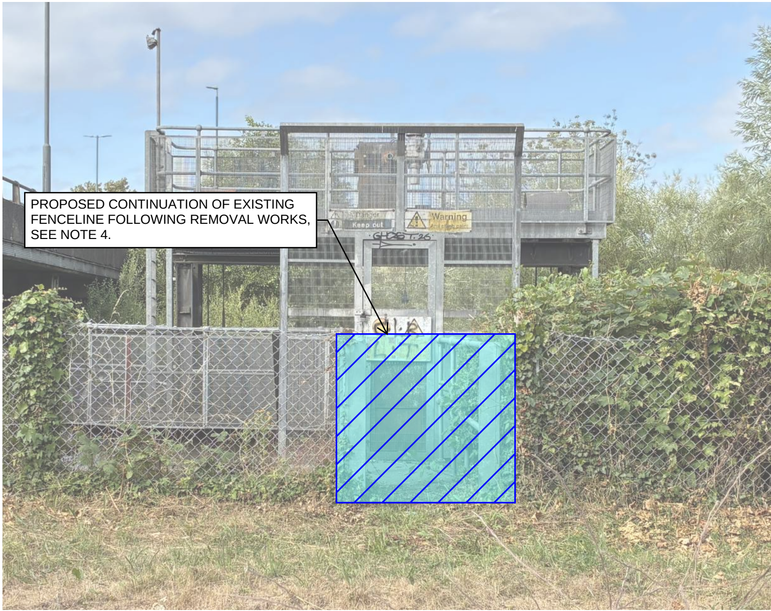
PHOTO 3: FENCE CONTINUATION AT SLUICE GATE ACCESS (NTS)
