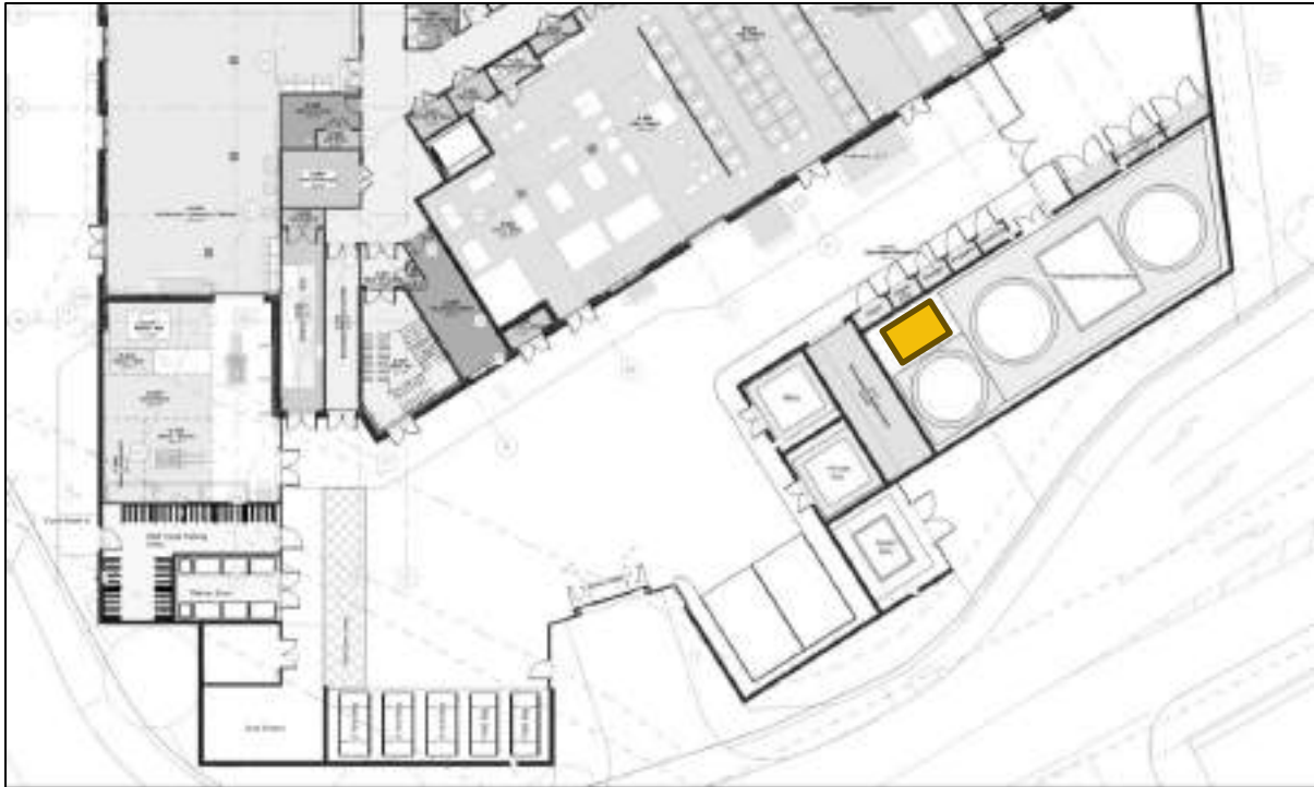
Figure 6: Emergency Generator Location in Service Yard (Image Source: Austin-Smith Lord)
