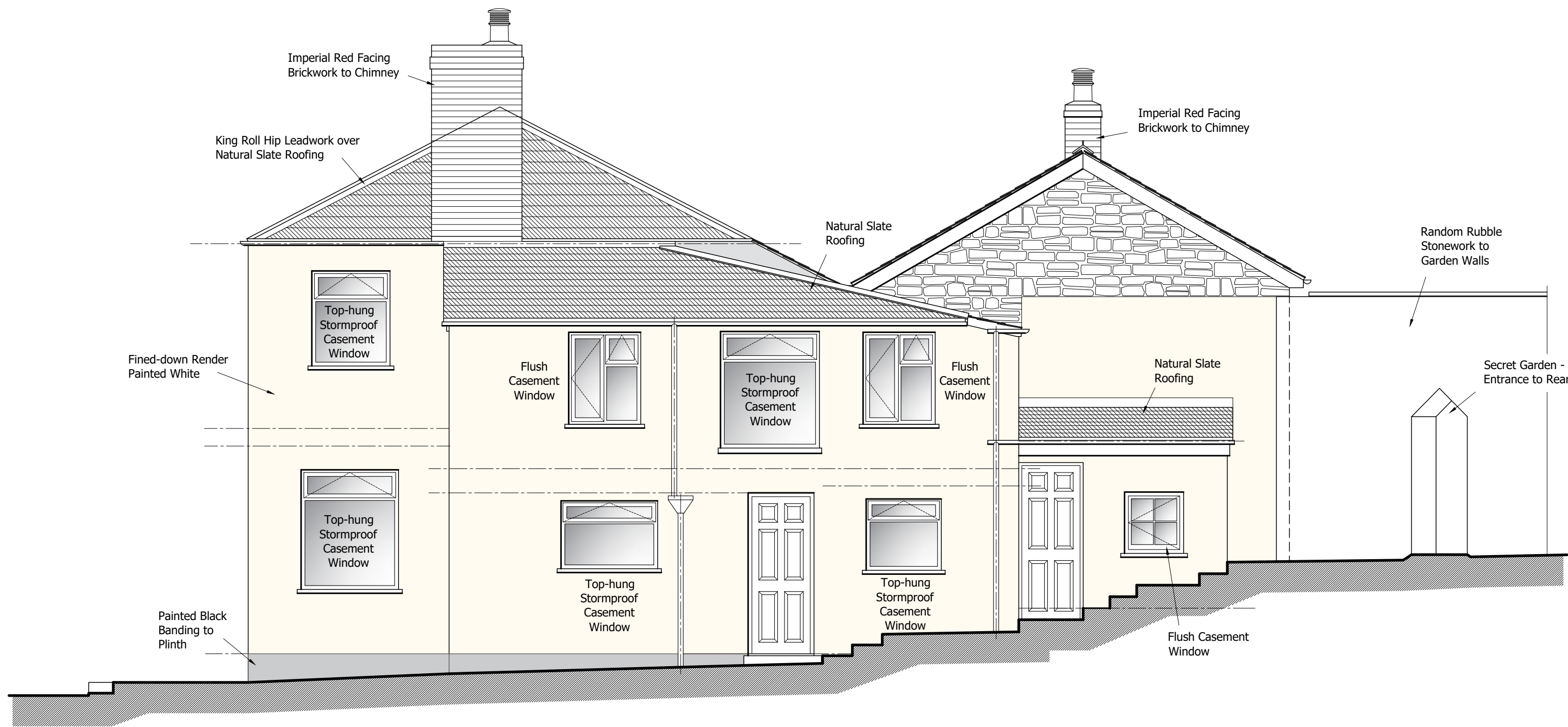
EXISTING SIDE ELEVATION WEST
