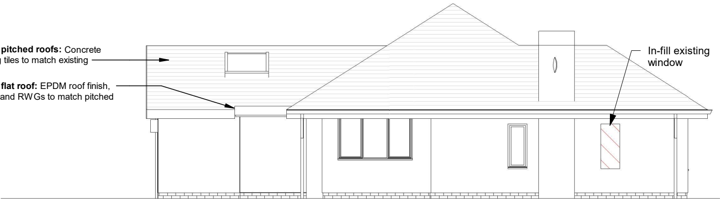
South West Elevation 1 : 100
