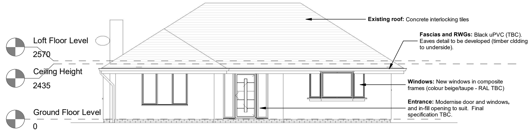
South East (Principal) Elevation 1 : 100
