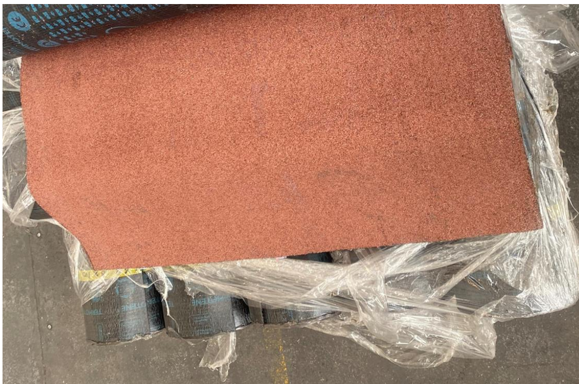
Bitumen walkway- Paralon ARD/S cap sheet in a terracotta red colour
