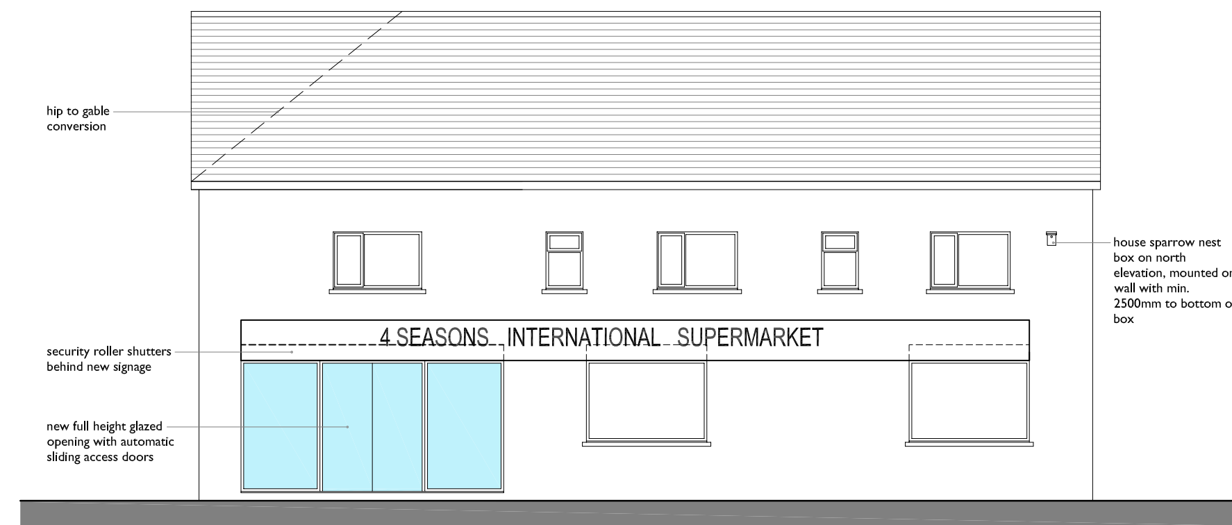
FRONT ELEVATION (WHARF ROAD)
