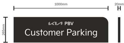
Sign 'E' Scale 1:25 Size: 1000mm x 265mm x 20mm Description: 20mm composite with anodised face to logo non illuminated Cap height of 'P' in 'Parking' = 90mm Logo Height = 35mm QUANTITY x2 Height from ground level: 1200mm
