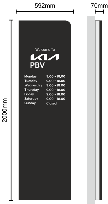
Sign 'C' Scale 1:25 Size: 592mm x 2030mm x 70mm Description: Wall Mounted welcome sign non - Illuminated Logo height = 75mm PBV height = 61mm Cap height of 'M' in 'Monday' = 34mm Height from ground level: 100mm
