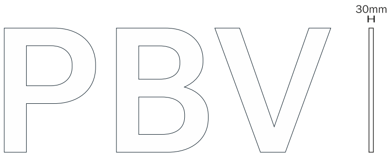
Sign B Scale 1:25 Size: 2227mm x 850mm x 30mm Surface mounted opal acrylic 'PBV' letters Height from ground level: 5428mm
