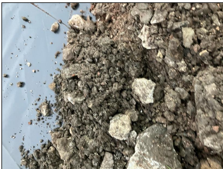
Figure 5-D: Made Ground at WLS02 between depths of 0.6 to 0.8m bgl
