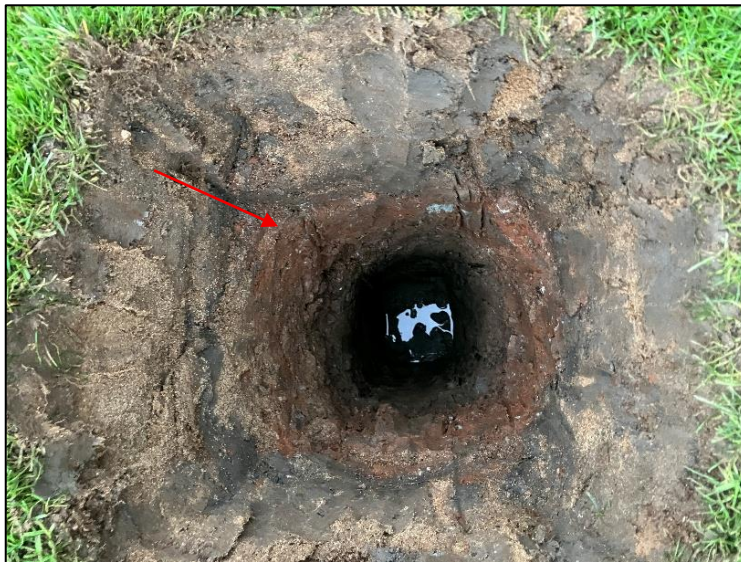
Figure 5-C: Layer of reddish brown Made Ground observed insitu at WLS04
