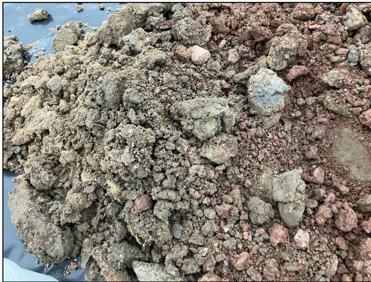
Figure 5-B: Made Ground from WLS05 between depths of 0.3 to 0.5 m bgl
