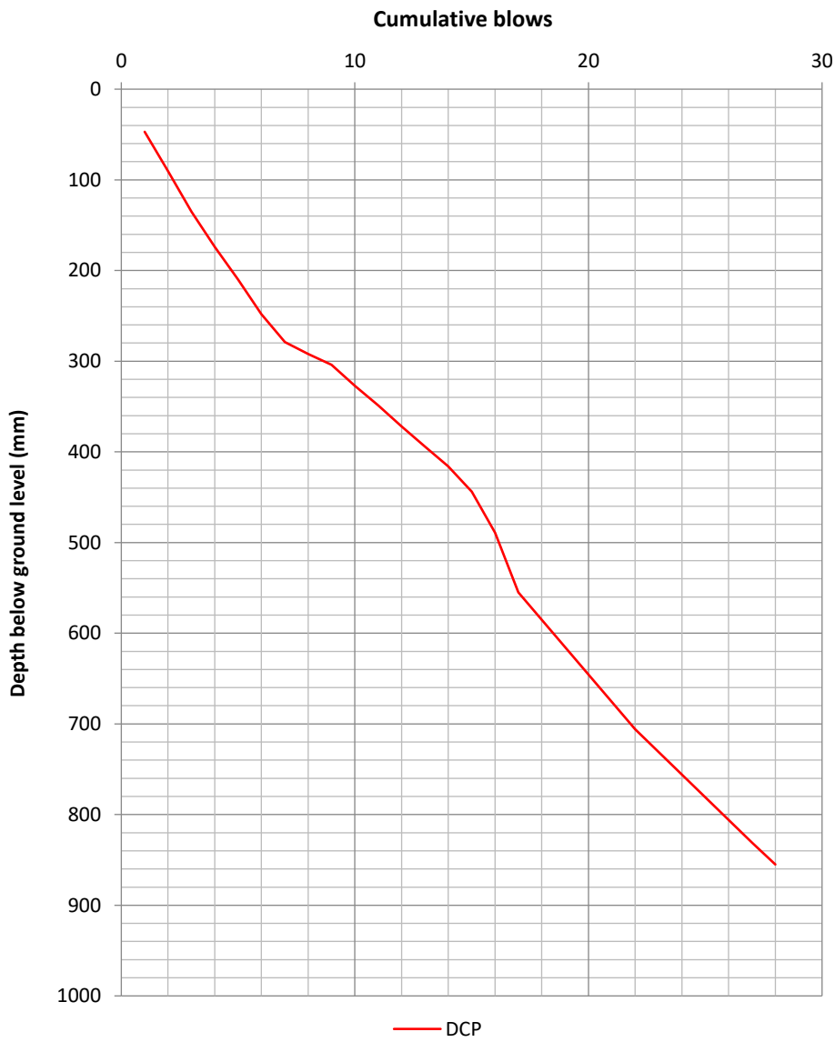
Plot showing number of blows against depth
