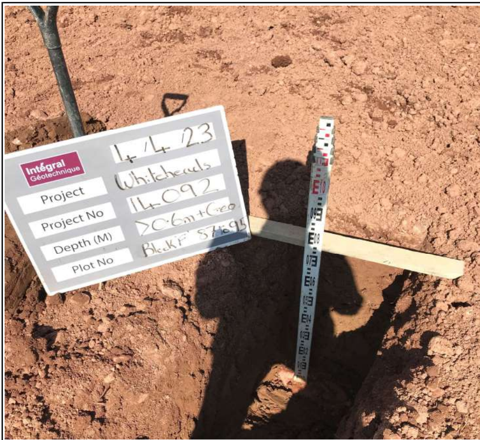
Block F (Plots 87 to 95) Excavation Trial Pit
