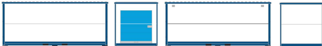
Type 3 – 2.4m x 6m unit – door on end
