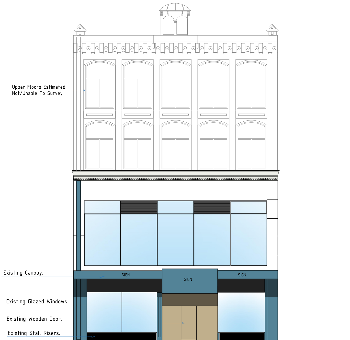
Existing As-built Front Elevation
