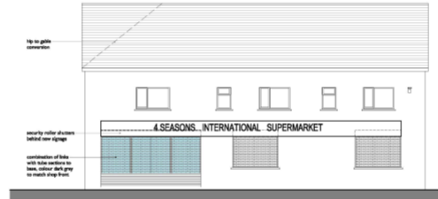
FRONT ELEVATION (WHARF ROAD) WITH SHUTTERS CLOSED
