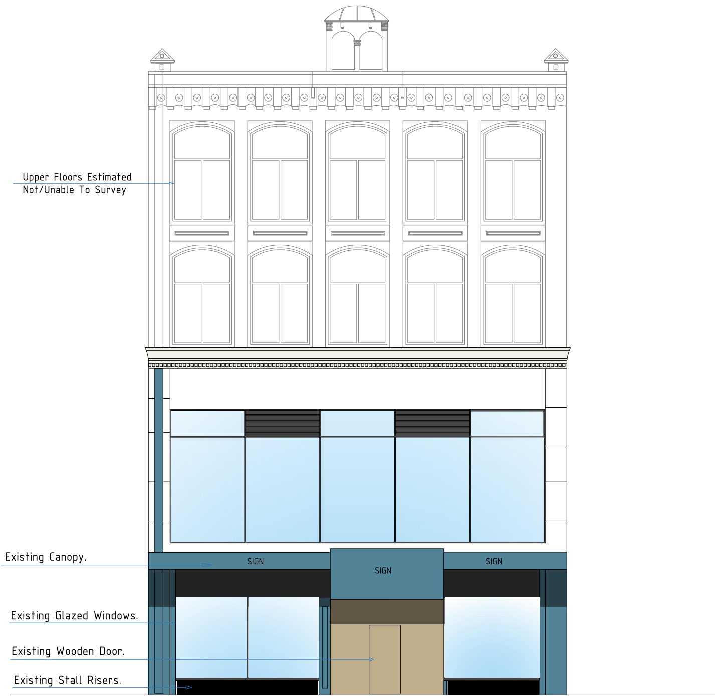
Existing As-built Front Elevation
