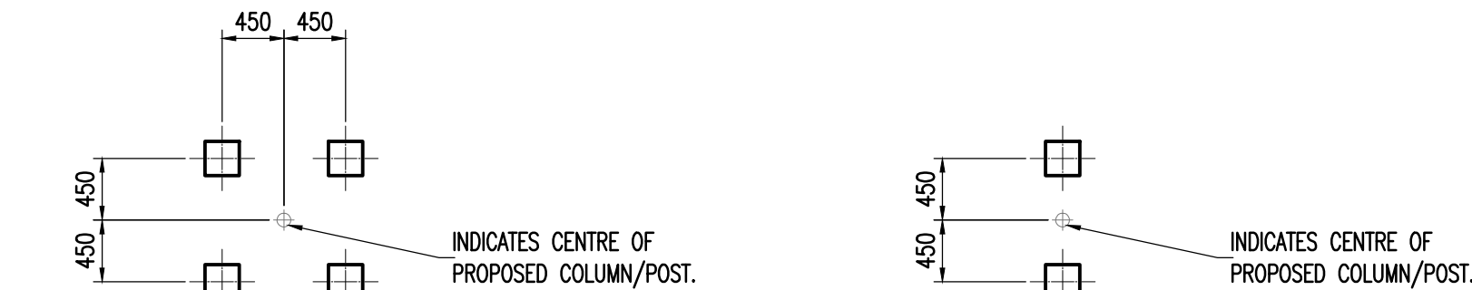
PILE CAP PC04 TYPICAL PILE SETTING OUT (1:50)
