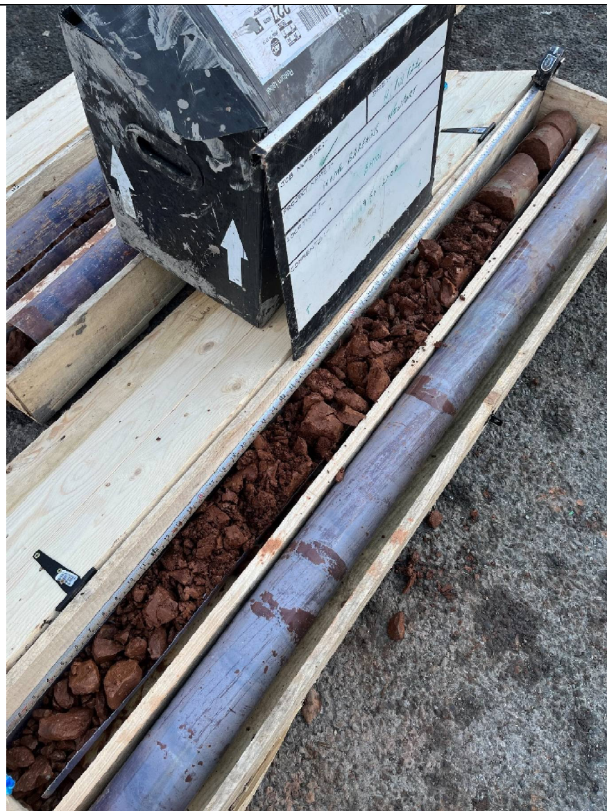
Plate 3: BH101 core run (19.50 -21.00m)
