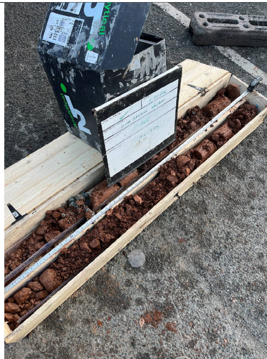
Plate 2: BH101 core run (18.00 -19.50m)
