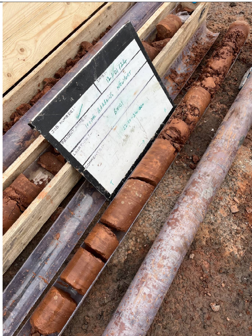
Plate 5: BH101 core run (22.50 -24.00m)
