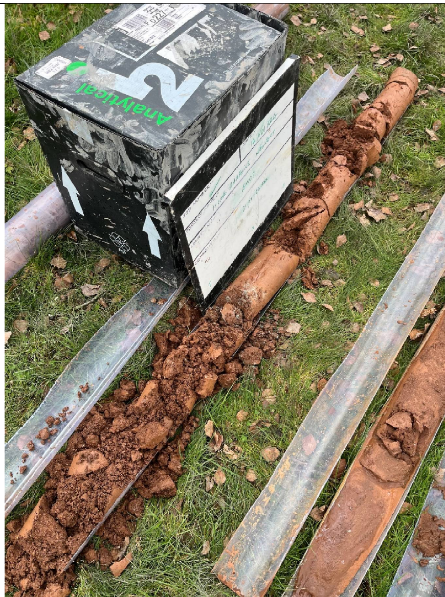
Plate 10: BH103 core run (21.00 -22.50m).
