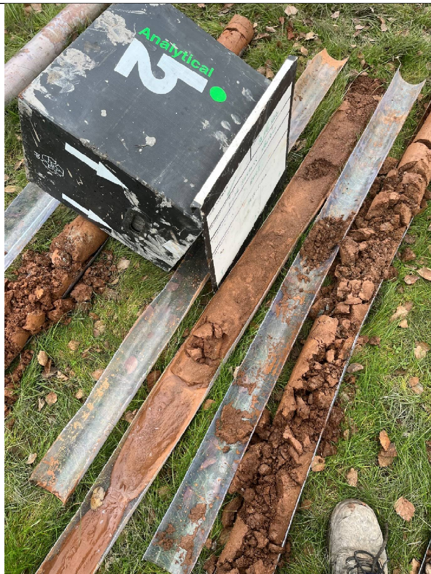
Plate 9: BH103 core run (19.50 -21.00m).
