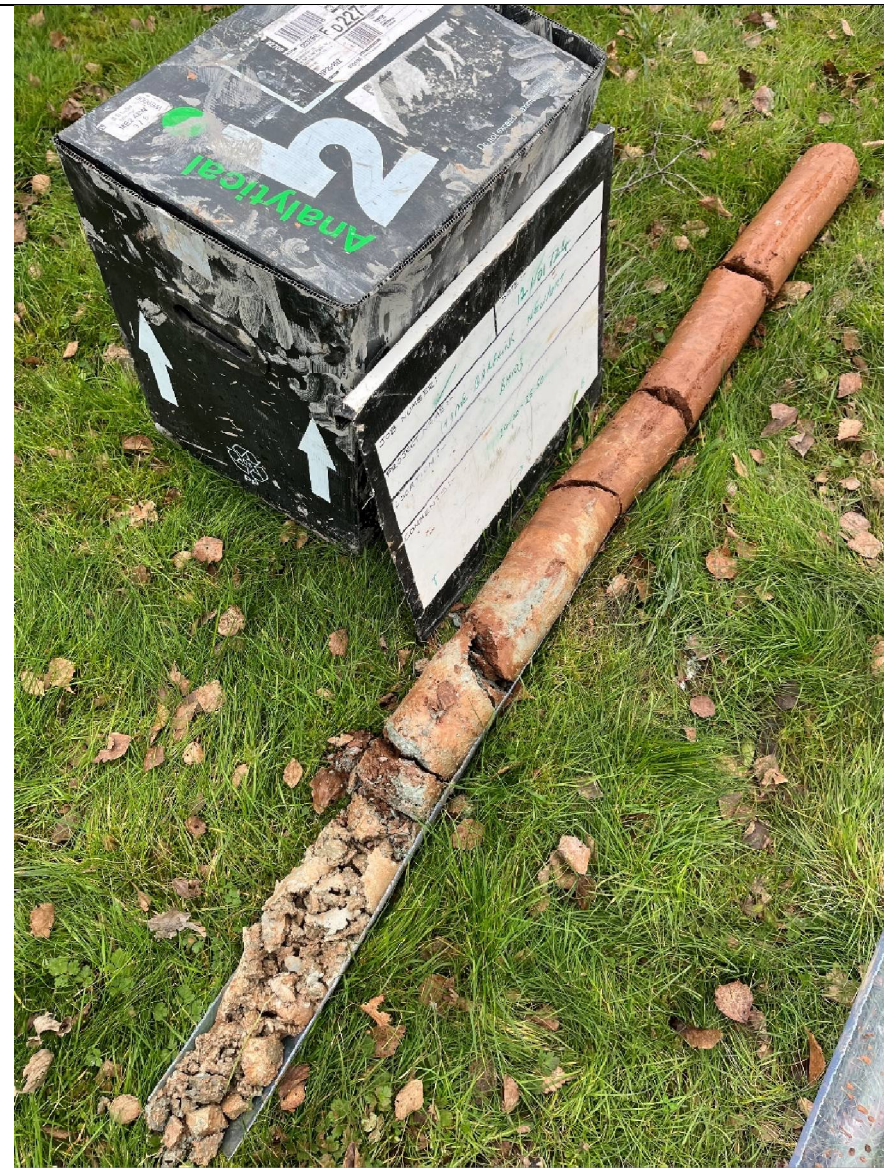
Plate 12: BH103 core run (24.00 - 25.00m).
