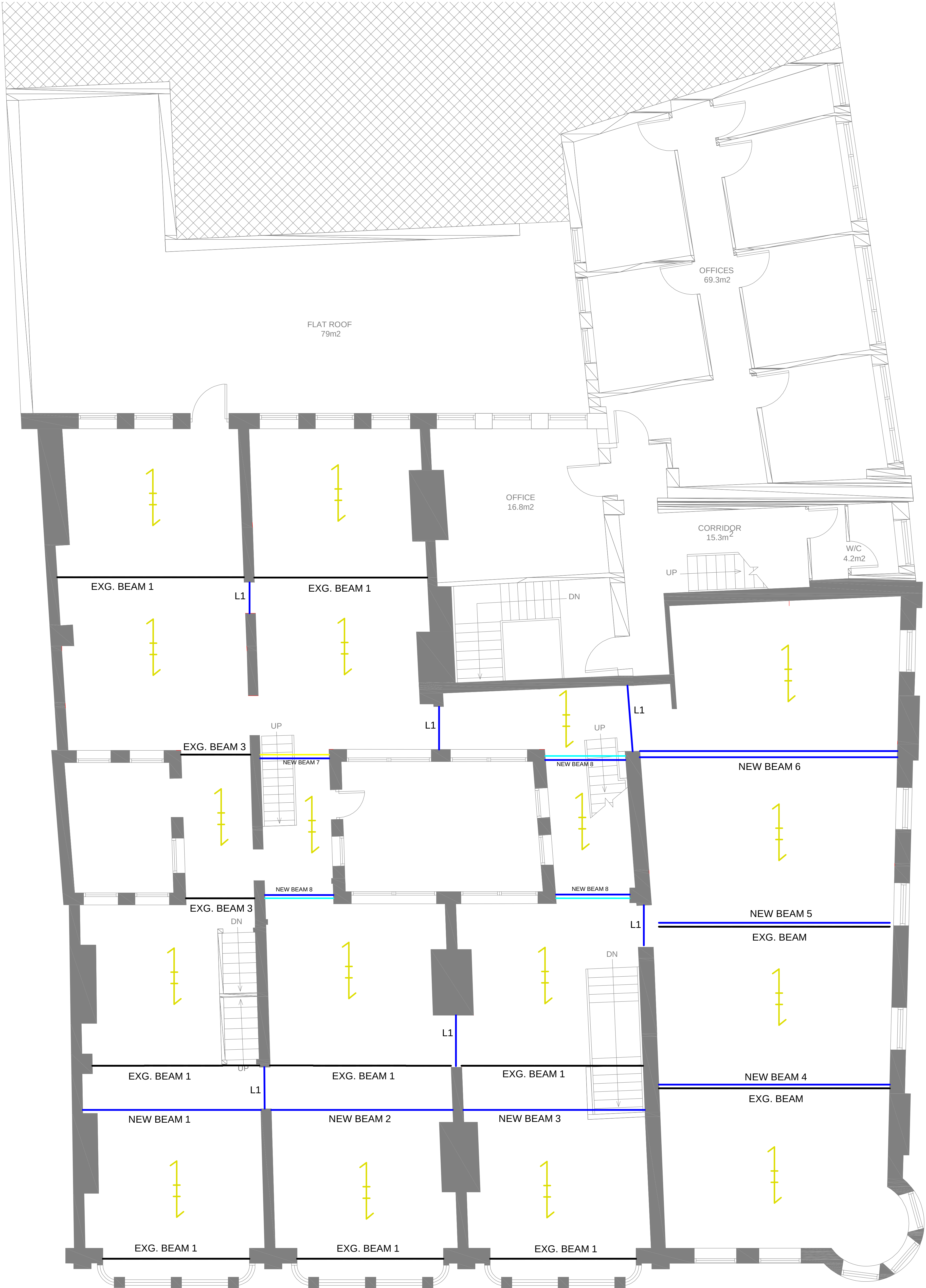
GENERAL ARRANGEMENT TOP OF FIRST FLOOR
