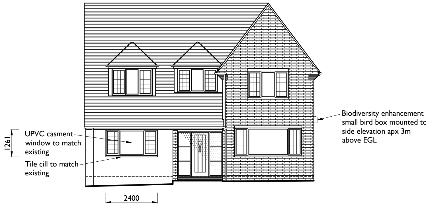
PROPOSED FRONT ELEVATION Scale 1:100
