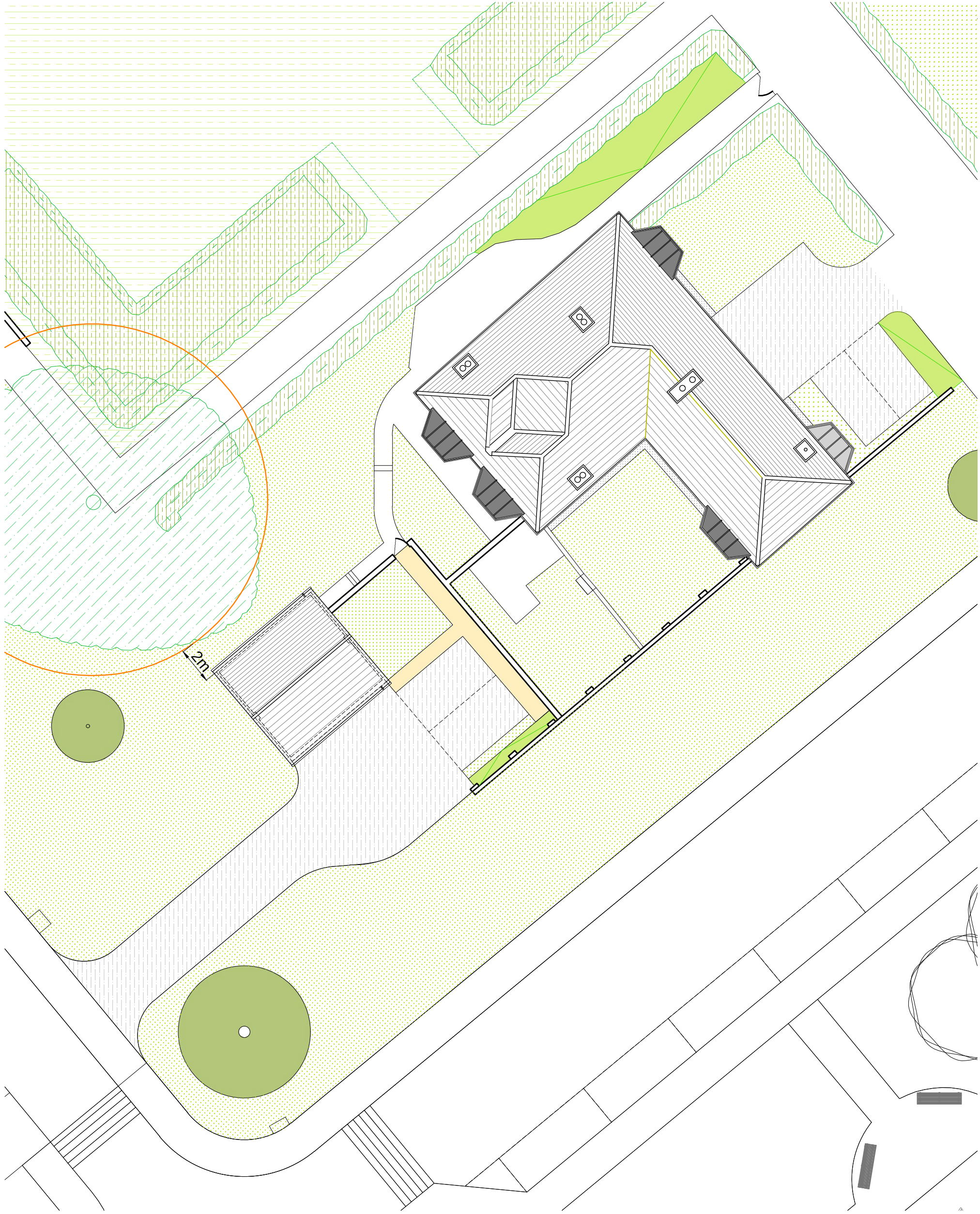
Proposed Principal Residence Site Plan (proposed double garage) Scale @ 1:200
