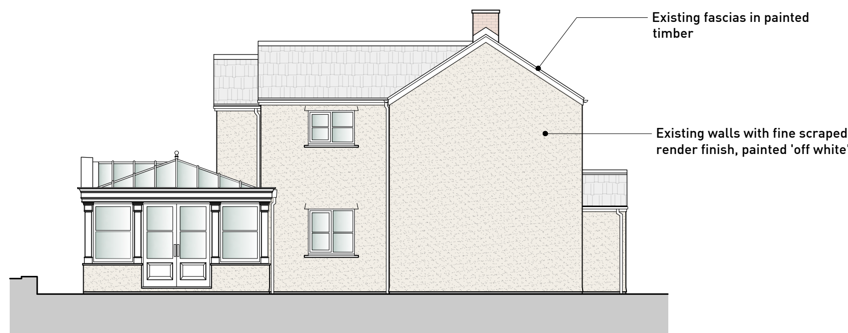
EXISTING SIDE ELEVATION - EAST Scale @ 1:100
