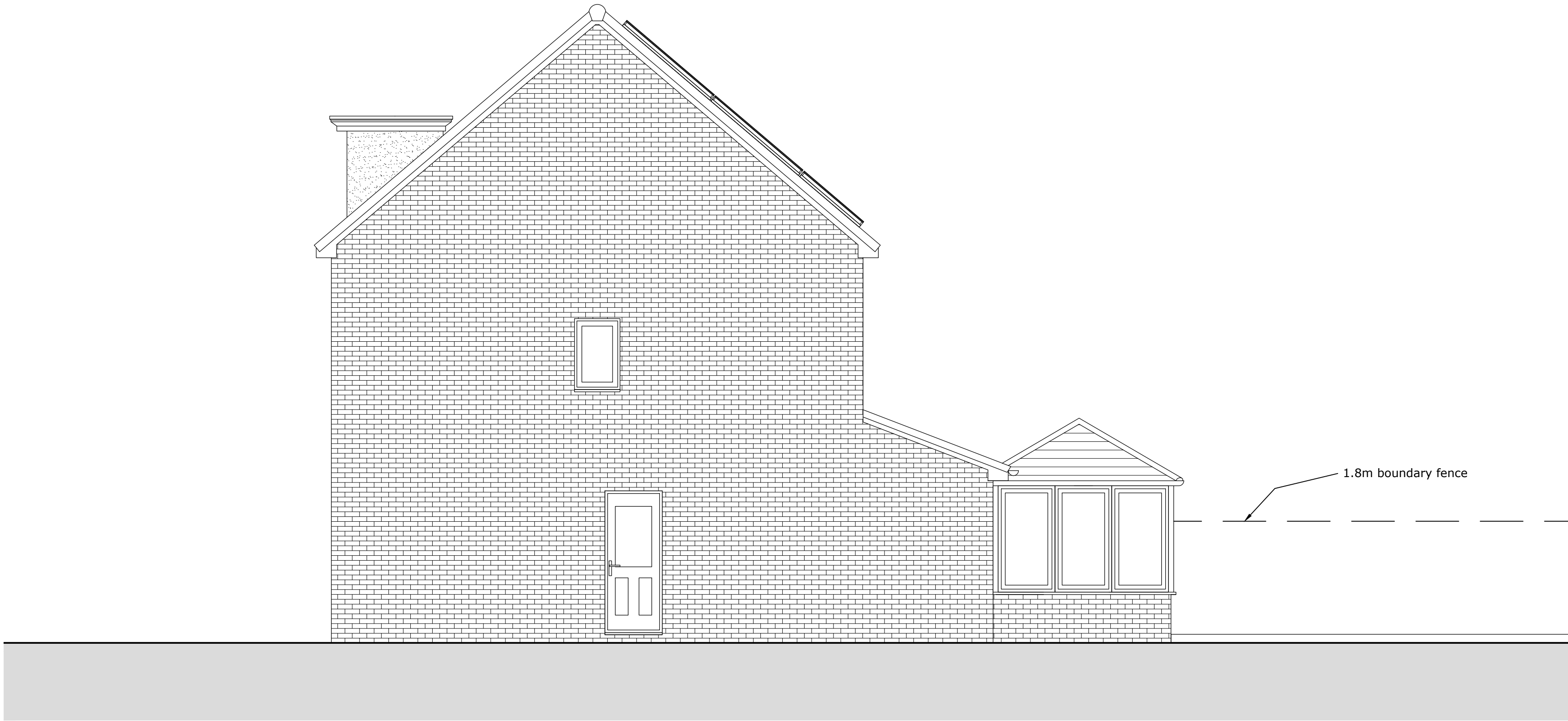
West Elevation as EXISTING 1:50
