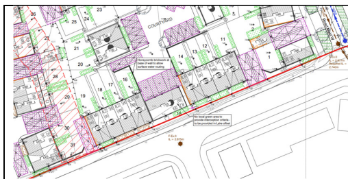
Engineering plan extract showing very high number of bioretention strips with 1 in 3 slopes to all front and rear gardens
