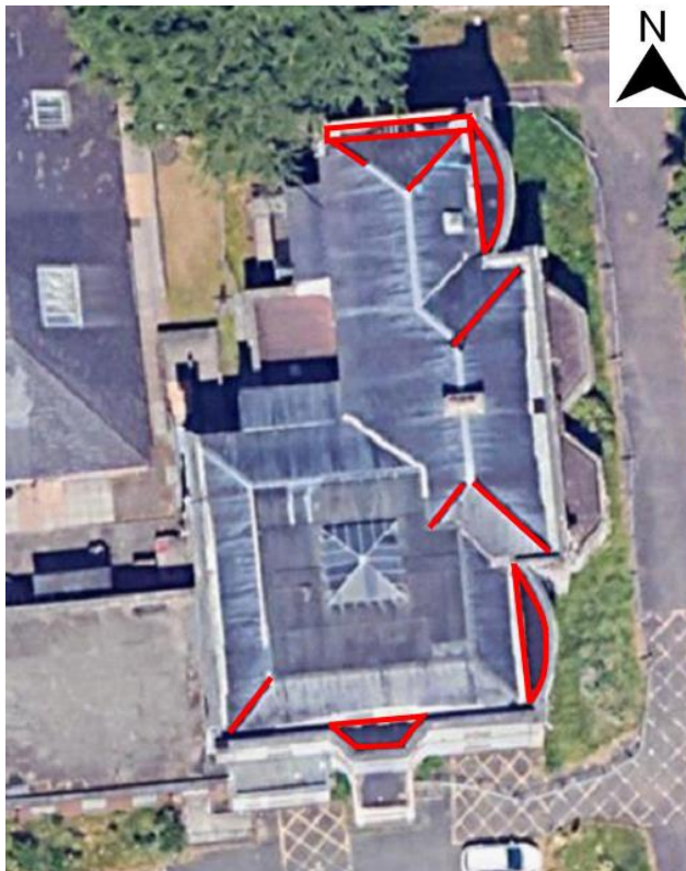
Left: roof plan showing extent of lead theft
