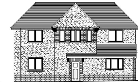
Existing Front Elevation
