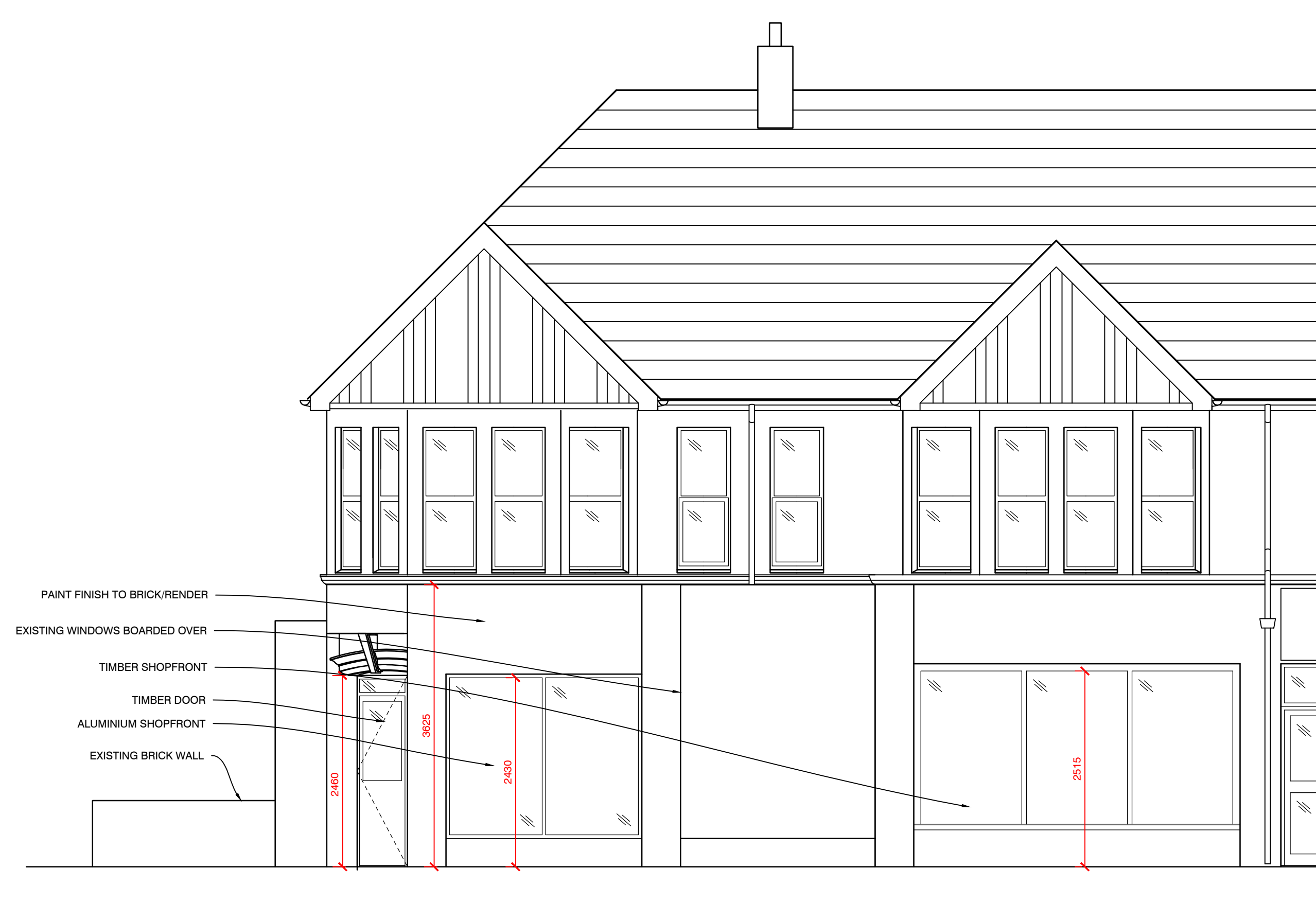
EXISTING NORTH SHOP FRONT ELEVATION A-A (1:50)
