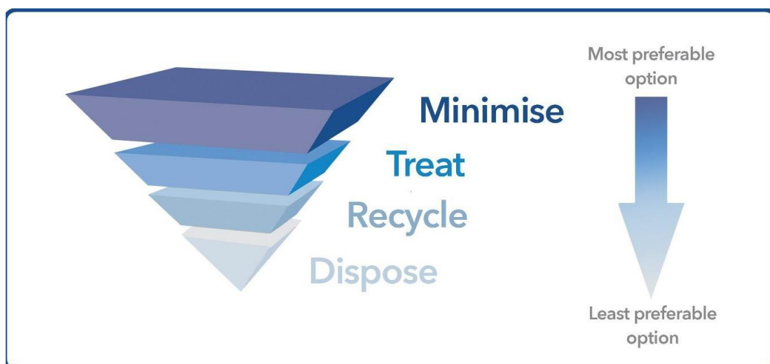
Figure 7.1 Water Treatment Hierarchy 3
