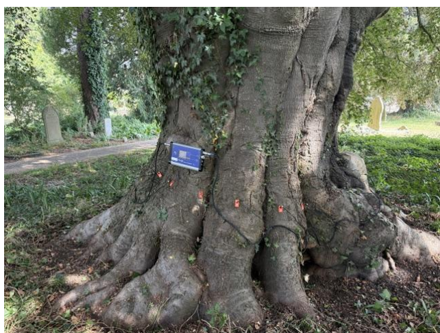
Picus 3 set up on tree for scanning.
